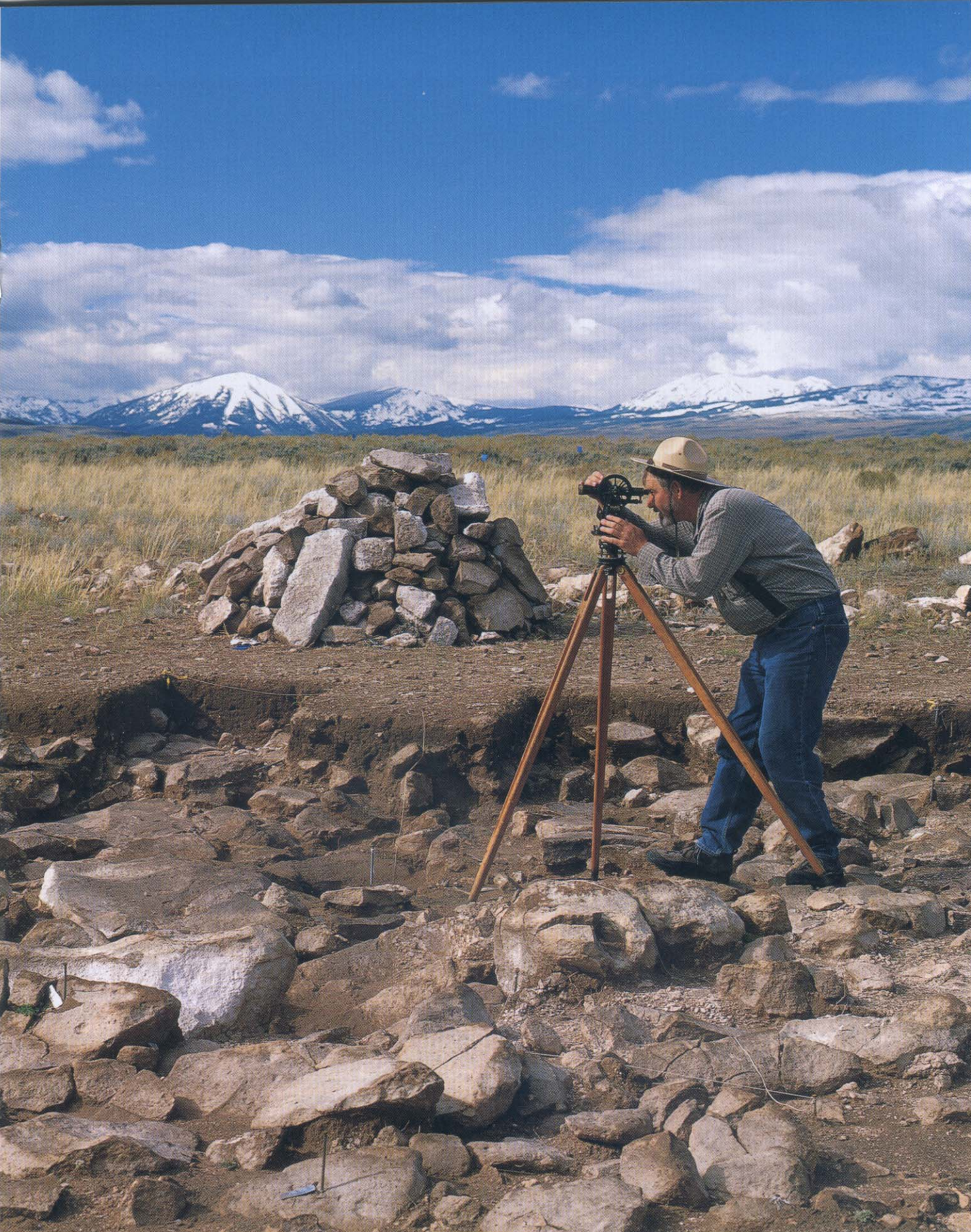
Mark Stiger illustrates mapping with an optical transit during an archaeology class on the Mountaineer site. The site, which is two miles from the Western State College campus, often serves as a classroom. The rocks from the foundation and walls of the Folsom house form the large pile in the center of the photograph.
